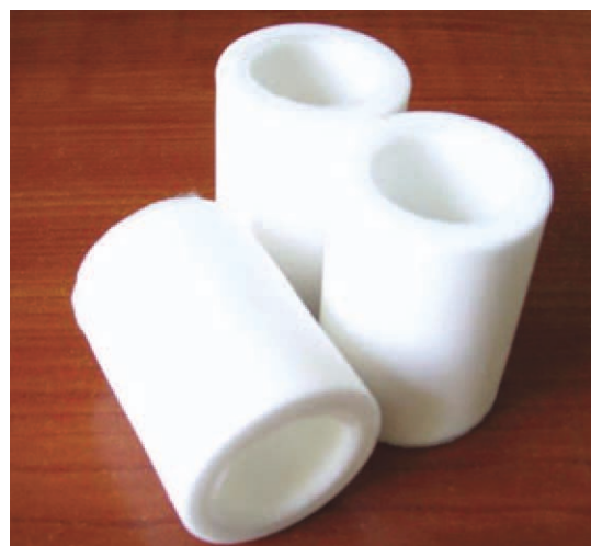
Figure 2 UHMWPE microporous product. [Color figure can be viewed in the online issue, which is available at wileyonlinelibrary.com .]
